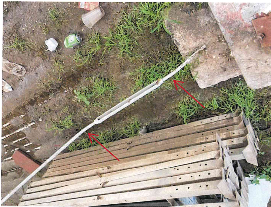
Figure 17 – Close-up photo showing bent/damaged cross-bracing rods
